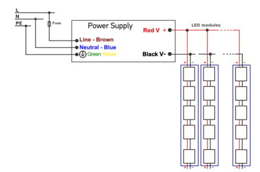
When there is a need to power more LED modules can use multiple PS powered in parallel by mains.
